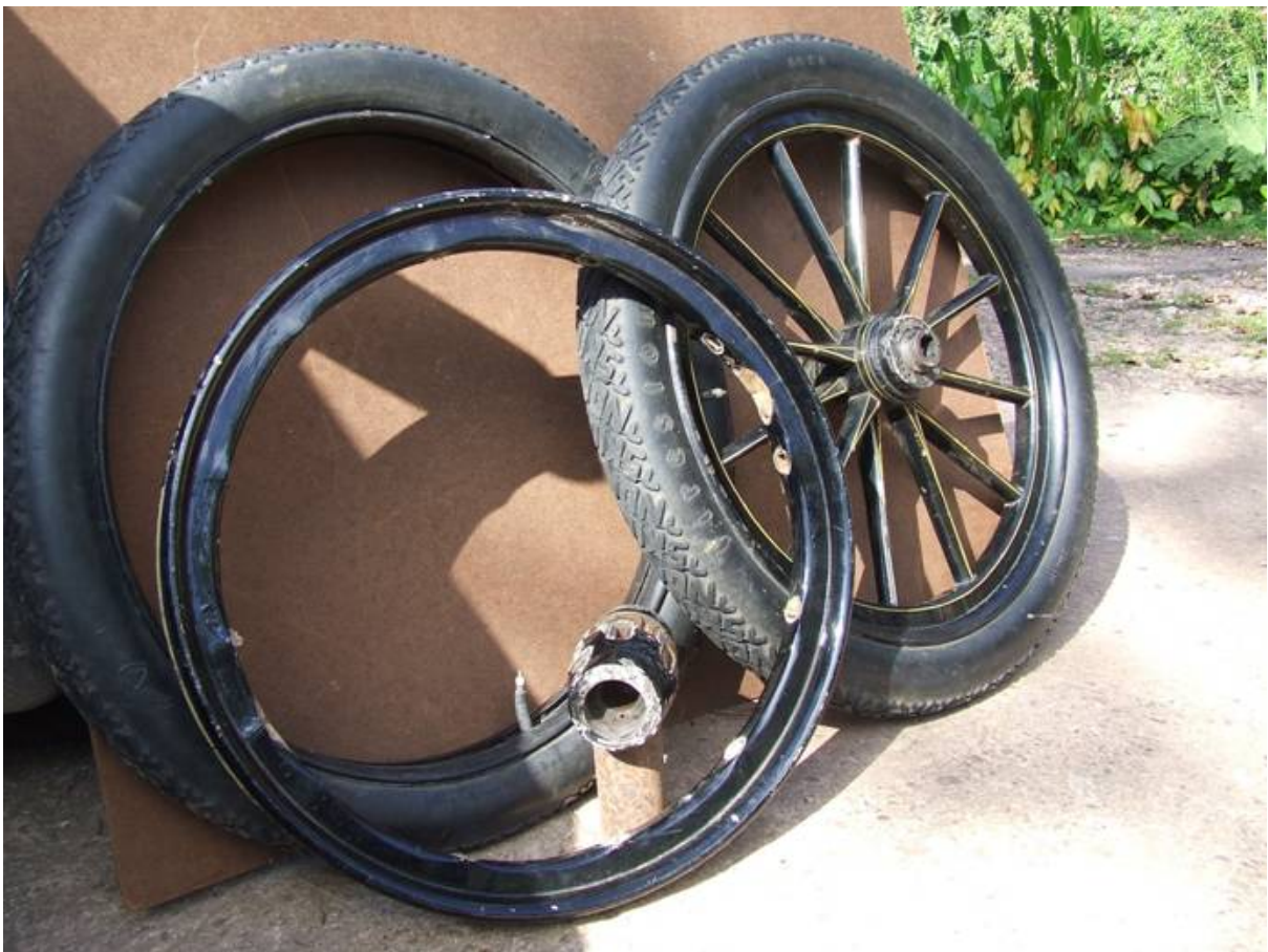
Figure 1 a damaged wheel, and a good one, from a 1902 Oldsmobile,
